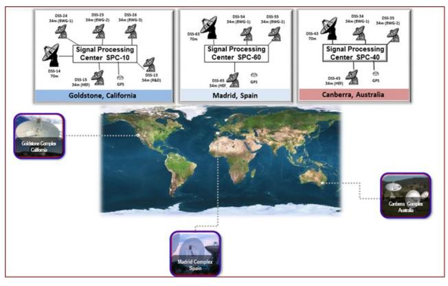
• The three sites, Goldstone (USA), Madrid (Spain), and Canberra (Australia) are spaced approximately 120 degrees apart in longitude to provide nearly continuous tracking coverage for missions above the Geosynchronous Earth orbit of 35,786 km (22,236 mi).
