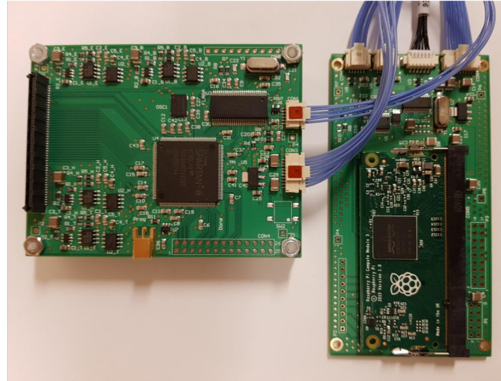
NODE FPGA board and CPU
