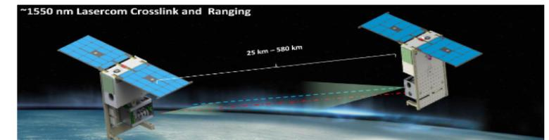
Leveraging previous investments by NASA STMD, STTR, AFRL UNP, and both universities, CLICK will demonstrate free space optical crosslinks with with picosecond timing accuracy (University of Florida), and precision pointing, acquisition, and tracking controls (MIT AeroAstro) in Low Earth Orbit.
