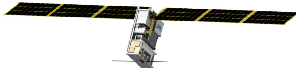
Lunar IceCube (6U CubeSat) in Flight Configurations
