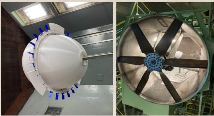
Half-Size Probe Wind-tunnel testing at NASA-LaRC in Virginia
