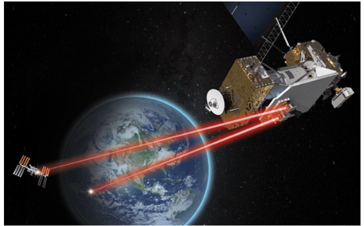
Launched in December 2021, the Laser Communications Relay Demonstration will demonstrate optical communications capabilities for future missions. Most spacecraft use radio frequency technology to communicate with Earth. Optical communications could increase bandwidth 10-100 times more than radio frequency. (Artist Illustration) Image Credit: NASA
