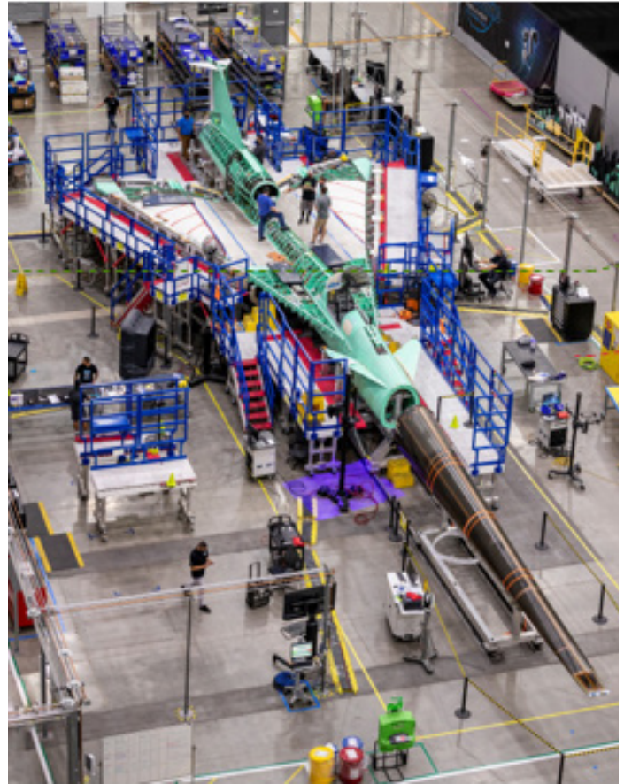
The X-59 QueSST (Quiet SuperSonic Technology) aircraft will fly at supersonic speeds above communities during the Low-Boom Flight Demonstration mission, generating sonic "thumps" instead of booms. Image credit: NASA/Lockheed Martin
