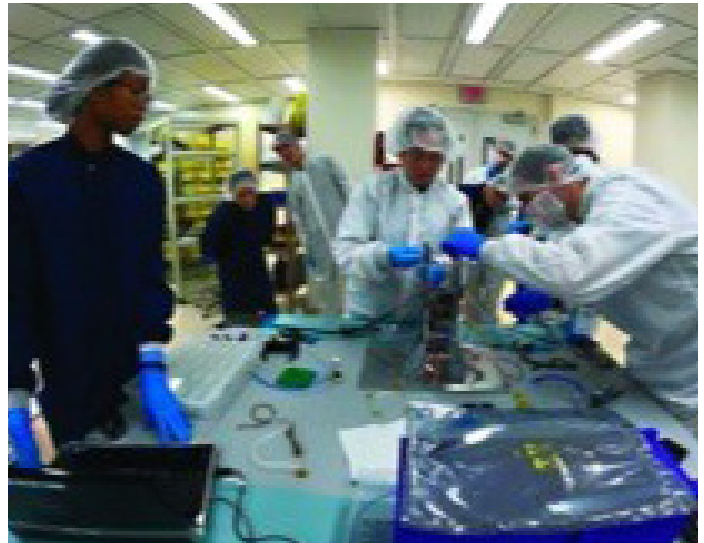
Hawaii Space Flight Laboratory undergraduate students, summer interns and engineers integrating the Neutron-1 3-U CubeSat in a cleanroom. NASA Space Grant, MUREP, and EPSCoR will continue to fund a wide spectrum of competitive student and institutional research opportunities to enable contributions to NASA's work in science and exploration. Image Credit: University of Hawaii at Manoa
