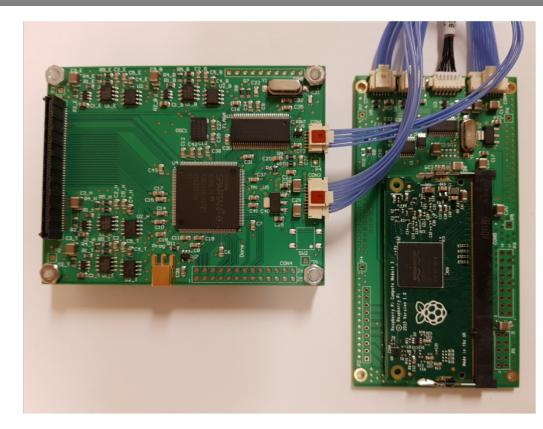
NODE FPGA board and CPU
